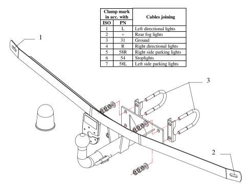
This towbar is designed to assembly in following cars: **SKODA 105** and **SKODA 120**, both produced since 1984 till 1990, catalogue no. **H 01** and is prepared to tow trailers max total weight **750 kg** and max vertical load **50 kg**.
